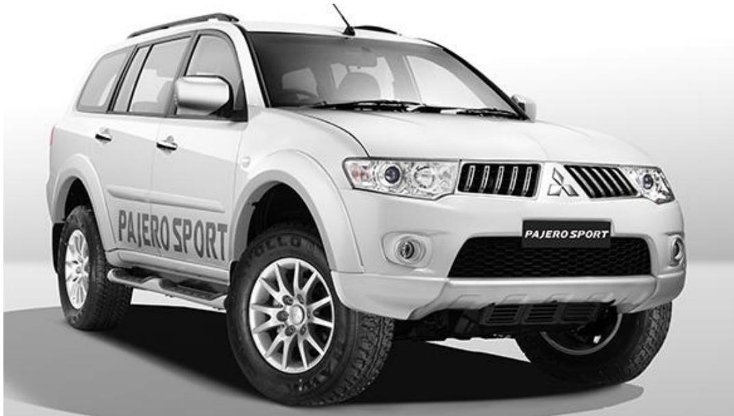
It comes with a super select 4WD system which allows one to choose between the 4x2 mode to increase fuel efficiency and three different 4x4 modes as per the terrain. Other features include a touch screen infotainment system, GPS navigation, rear view camera, rear spoiler, body colored bumpers, mud guards and Anniversary Edition decals.
