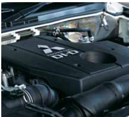
The 3.2 l diesel engine is turbocharged
