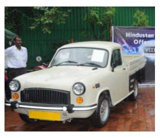
Talking about the vehicle, the 800kg payload pickup is available in BS3 (diesel) and BS4 (CNG fuel) versions. The vehicle can also be ordered as a drive-away chassis (DAC).
